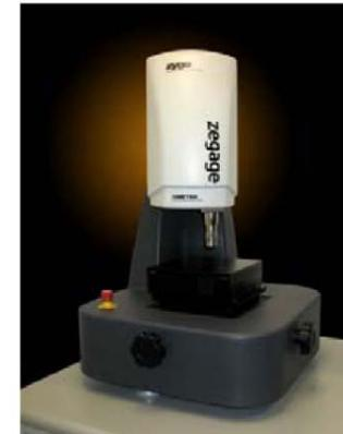
SEE 3-D replicate is examined with white light interferometer
